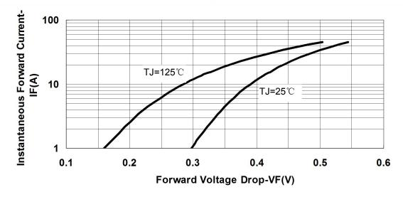
Fig.3-Typical Instantaneous Forward Voltage Characteristics
